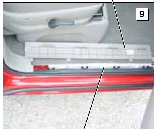
Route power supply cable through door sill area.
