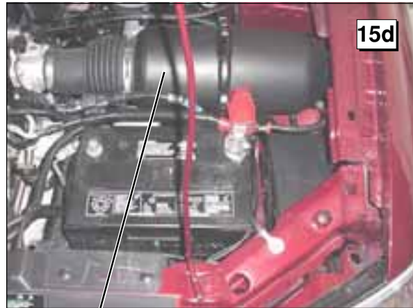
Midsection of Intake Duct
