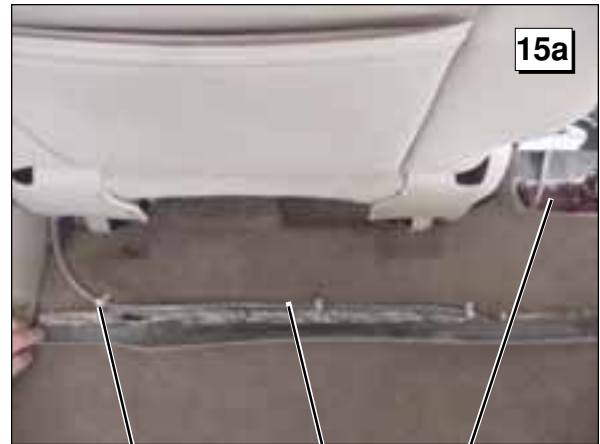
Plastic Cable Clip with Self Tap Screw Seam in Carpet with Power Harness Void in Carpet
