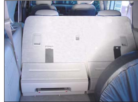
View from Rear of Modified Third Row Seat (in folded position)
