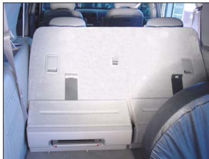
View from Rear of Modified Third Row Seat (in folded position)
